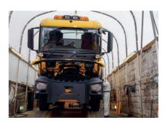
A key autumn task for gritters employed by councils is calibration, points out Lupton at Econ Engineering. It - along with gritting records - safeguards the operator and customer in the event of an accident. Calibration is also useful as a scheduling check and balance. The gritter can't be operated until it has been calibrated,
